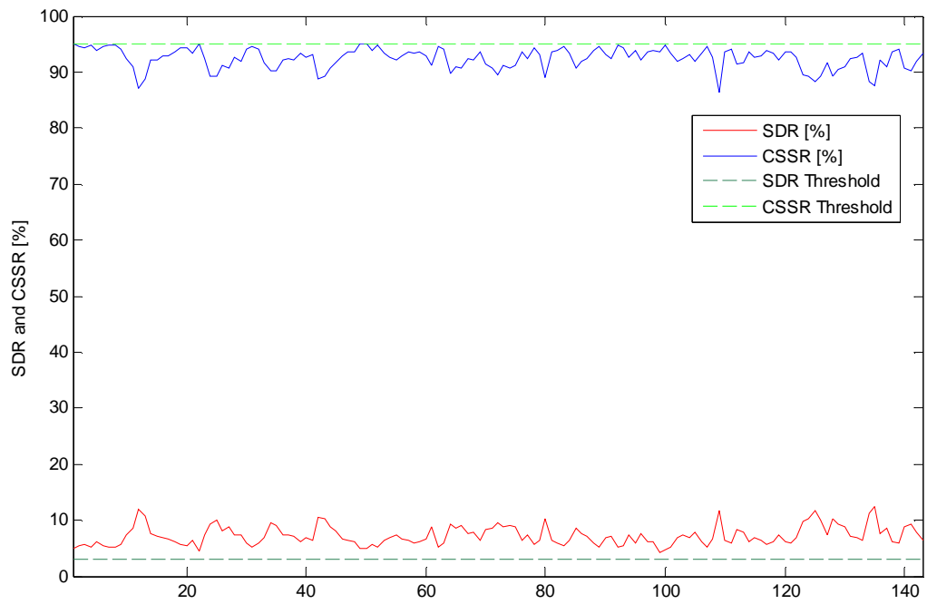
Figure D.10 BS 17 – R_{SDCCH_D} and R_{CS_S} performance analysis: correlation value of -98.35%.
