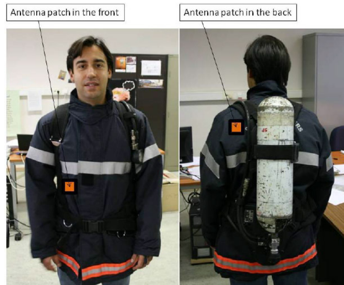
Figure 3.5. Wearable antennas integrated into a firefighter jacket (extracted from [VTHR10]).
