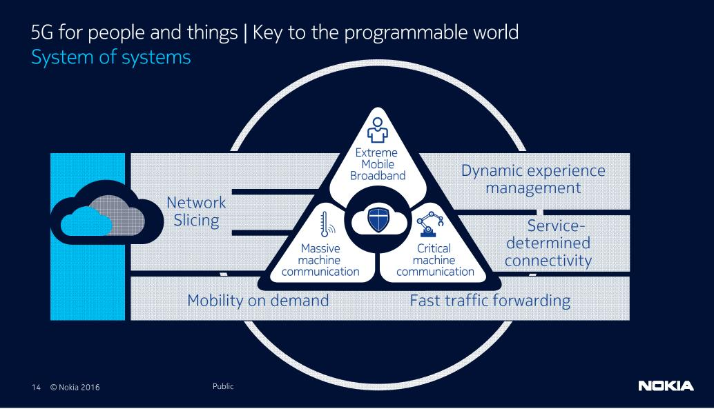
Network Slicing | Optimized service delivery for heterogeneous use cases Multiple independent instances on one physical network
