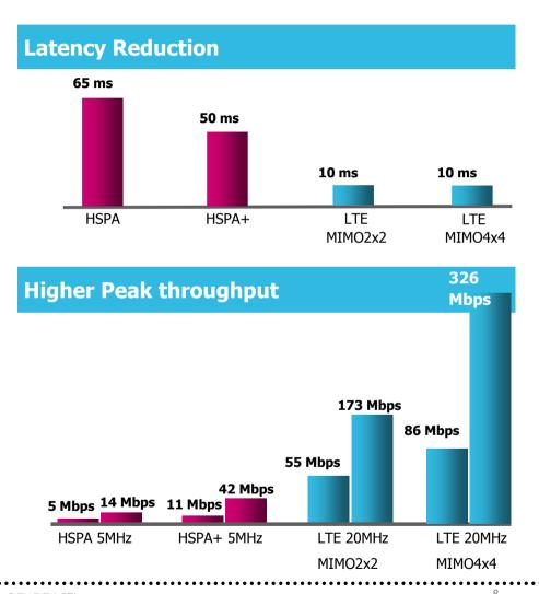
Low latency enables fast channel adaptation therefore allowing high speed applications
