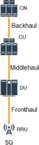
Figure 2.5 – 5G O-RAN implementation (adapted from [34]).
