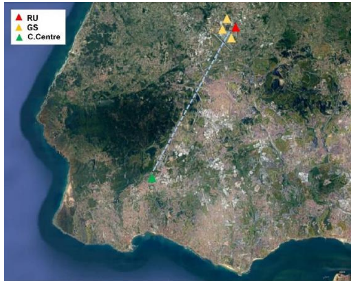
Figure 4.7 – Map positions of the WAM System’s GSs, Control Centre (EMFA) and Airbase N o .1 with a representation of a straight-line connection (11 km) between the Control Centre and the RU node.
