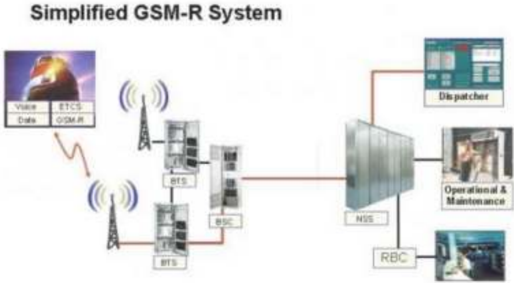
Figure 1.3 – Simplified GSM-R system (extracted from [GSMR23]).
