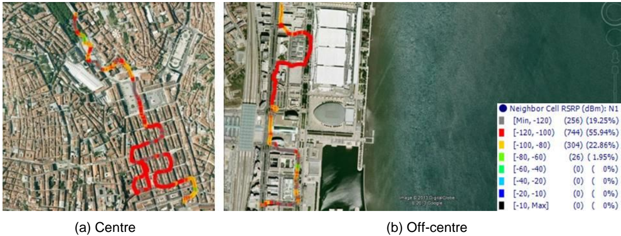
Figure F.7. Highest measured neighbour cell RSRP in the 2 600 MHz band for centre and off-centre areas.
