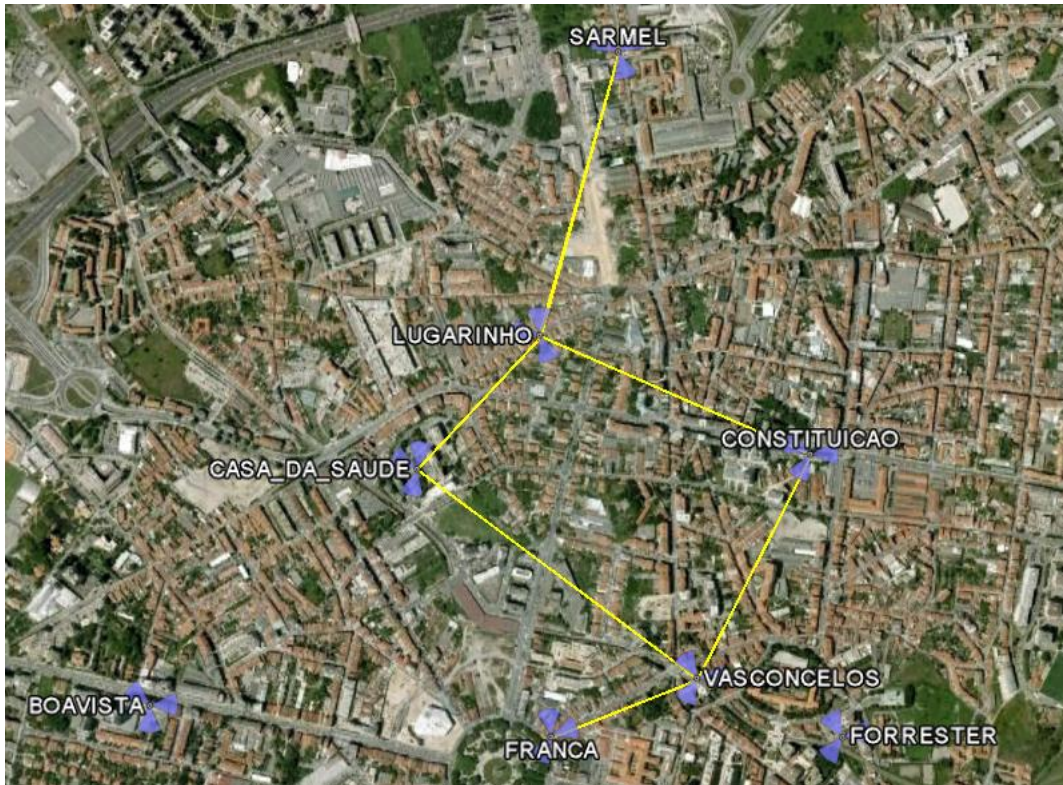
Figure G.3. Inter-BS distance, measured as the distance to the closest detected cell, for the Urban environment (extracted from [GoEa11]).
