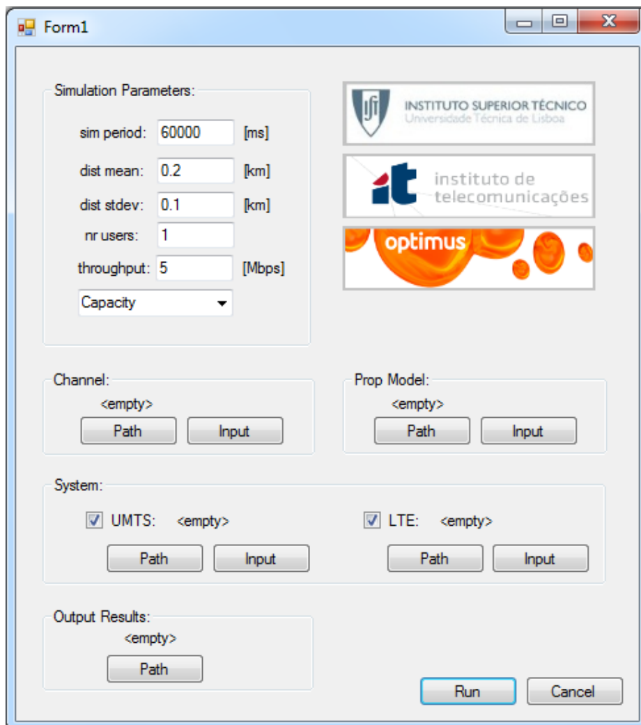
Figure E.1. Main simulator window: simulation parameters, channel, propagation model, systems' and output results path definition..
