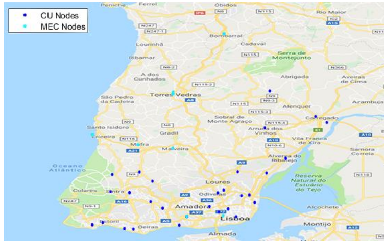
Figure N.4. CU and MEC node state for a maximum 5 ms E2E maximum latency in Lisbon.
